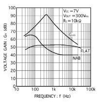
Voltage gain vs. frequency Fig.4
