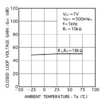
Closed loop voltage gain vs. Fig.7 ambient temperature
