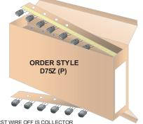
FIRST WIRE OFF IS COLLECTOR ADHESIVE TAPE IS ON BOTTOM SIDE FLAT OF TRANSISTOR IS ON TOP
