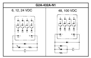
Note: Do not reverse the polarity of the coil of DC Relays that have a built-in indicator or diode.
