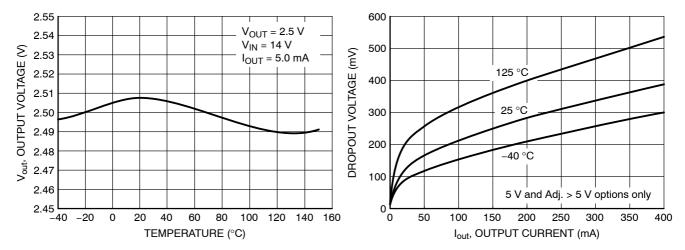
Figure 5. 2.5 V Output Voltage vs Temperature
