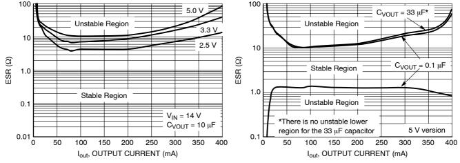
Figure 7. Output Stability with Output Voltage Change
