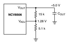
Figure 14. Adjustable Output Voltage
