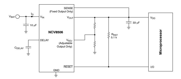
Figure 1. Application Diagram
