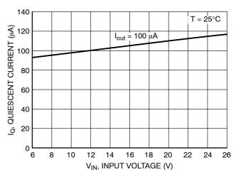
Figure 11. Quiescent Current vs Input Voltage
