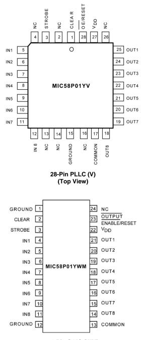
24-Pin SOIC (WM) (not pin compatible with MIC5801YWM)
