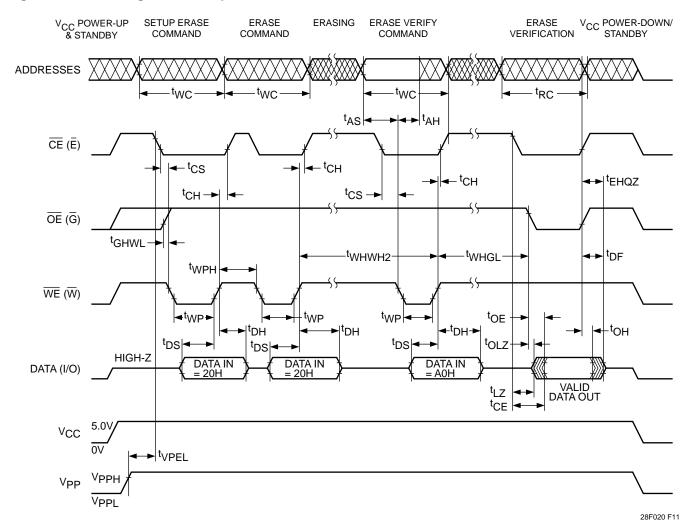
Figure 5. Chip Erase Algorithm<sup>(1)</sup>
