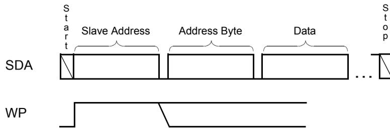
Figure 27. DCP "Wiper Position" Timing
