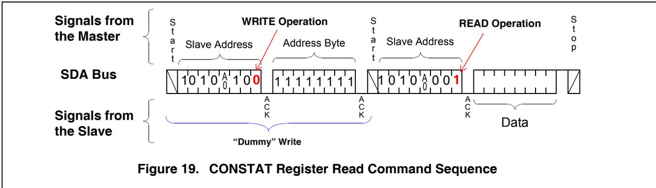
Figure 19. CONSTAT Register Read Command Sequence
