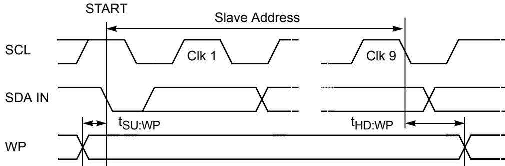
Figure 26. Write Protect (WP) Pin Timing
