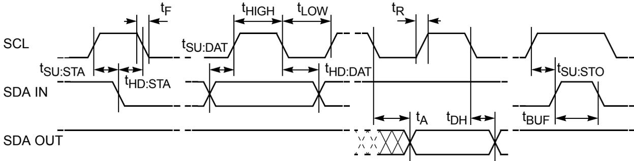
Figure 23. Physical Device Address ( $A_0$ ) Pin Timing
