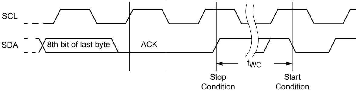
Figure 25. Write Protect (WP) Pin Timing During Slave Address
