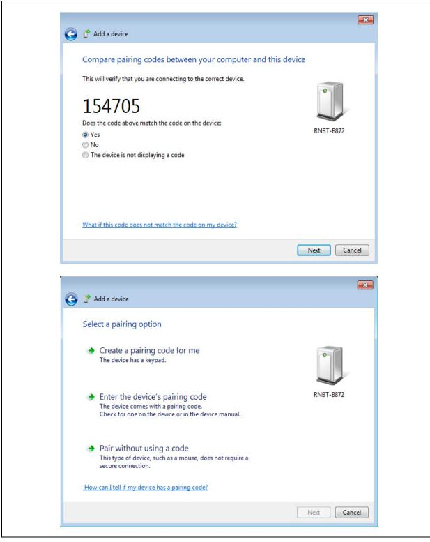
When the Bluetooth device manager completes pairing, it issues a message that the Bluetooth device is installed on COMX where COMX is unique to the used host computer. In some cases, the Bluetooth device manager creates two COM ports; in this case, *only* use the COM port labeled as outgoing. Figure 2-7 shows an example of COM port settings.
