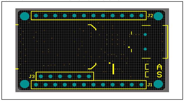
FIGURE A-4: RN41/42 EVALUATION BOARD BOTTOM SILKSCREEN
