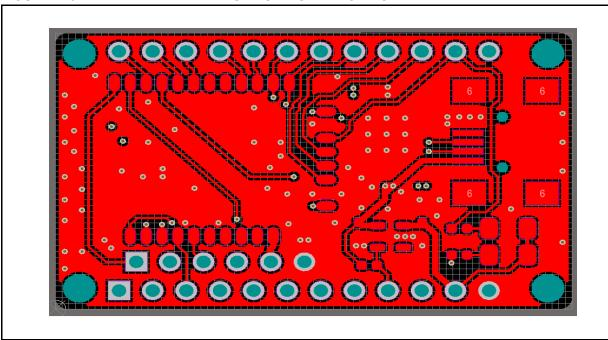
FIGURE A-6: RN41/42 EVALUATION BOARD BOTTOM COPPER
