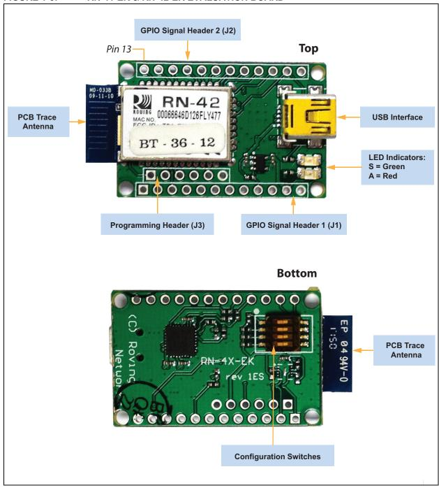
Note: Figure 1-3 shows the RN-42-EK board. This figure is similar to RN-41-EK board.
