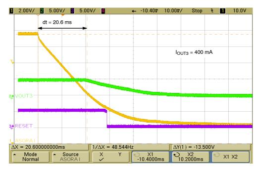
Figure 29. Output Response of LDO3 to Loss of Vin-B
