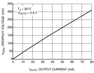
Figure 16. Dropout LDO2 vs Output Current
