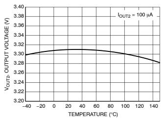
Figure 13. Output Voltage LDO2 vs
