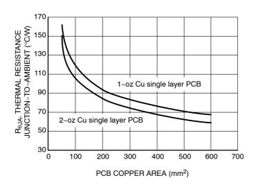
Figure 20.  $R_{\theta JA}$  vs. Copper Area
