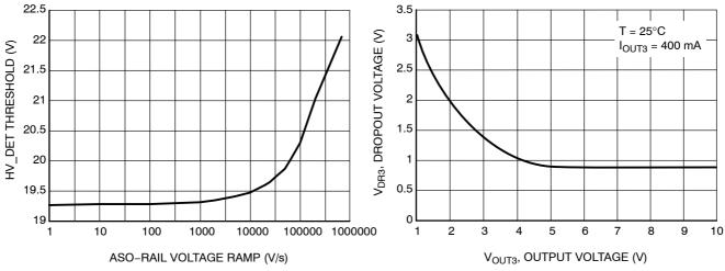
Figure 18. HV-DET Threshold vs. dV/dt
