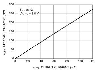
Figure 15. Dropout LDO1 vs Output Current
