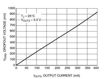
Figure 17. Dropout LDO3 vs Output Current
