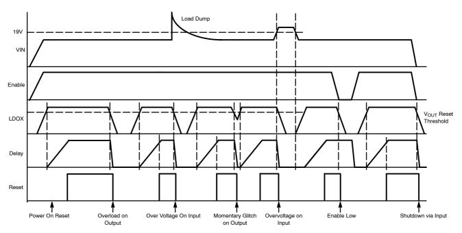
Figure 5. NCV8612B Reset Timing Diagram
