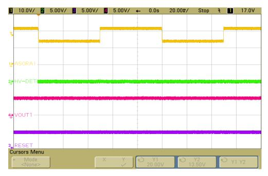
Figure 32. HV-DET Response to High Voltage - VBAT-MON Left Open
