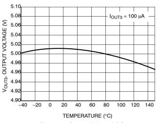
Figure 14. Output Voltage LDO3 vs
