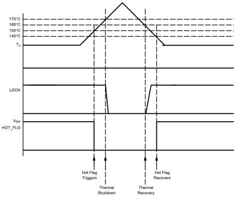
Figure 9. Thermal Shutdown Timing Diagram
