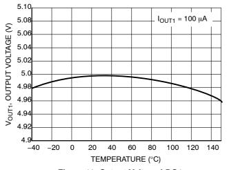
Figure 12. Output Voltage LDO1 vs
