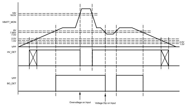
Figure 8. Warning Circuitry Timing Diagram
