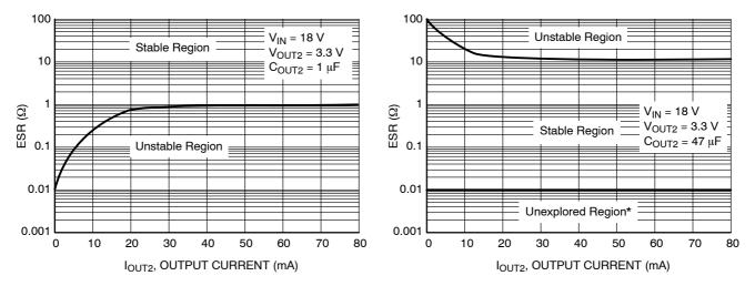
Figure 24.  $C_{OUT2}$  ESR Stability Region – 1  $\mu$ F Figure 25.  $C_{OUT2}$  ESR Stability Region – 47  $\mu$ F \*The min specified ESR is based on Murata's capacitor GRM31CR60J476ME19 used in measurement. The true min ESR limit might be lower than shown.
