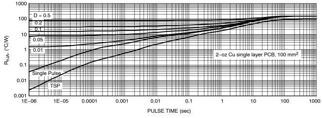
Figure 21.  $R_{\theta JA}$  vs. Duty Cycle
