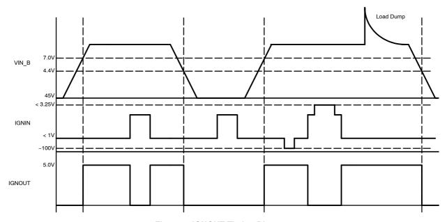
Figure 6. IGNOUT Timing Diagram
