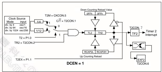
Figure 16. 16-Bit Auto-reload Up/Down Counter
