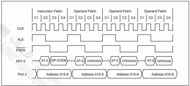
Figure 6: Four Cycle Instruction Timing
