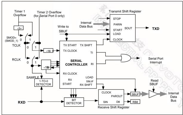
Figure 21: Serial Port Mode
