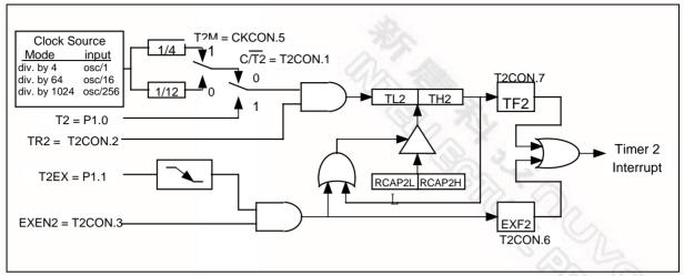
Figure 15. 16-Bit Auto-reload Mode, Counting Up
