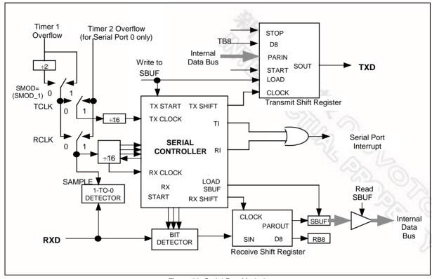
Figure 23: Serial Port Mode 3
