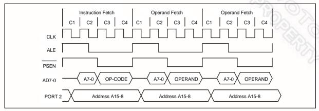
Figure 5: Three Cycle Instruction Timing
