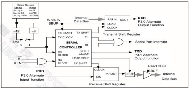
Figure 20. Serial Port Mode 0
