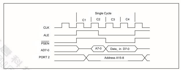
Figure 3: Single Cycle Instruction Timing
