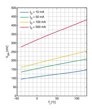
Guaranteed Dropout Voltage  $V_{\rm DR}$  versus Output Current  $I_{\rm Q}$
