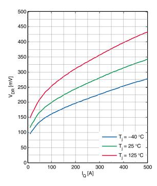
Dropout Voltage  $V_{\text{DR}}$  versus Junction Temperature  $T_{\text{j}}$
