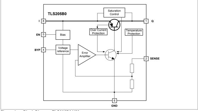
Figure 1 Block Diagram TLS205B0 V50
