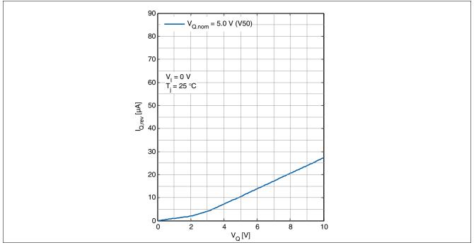
Figure 7 Reverse Output Current
