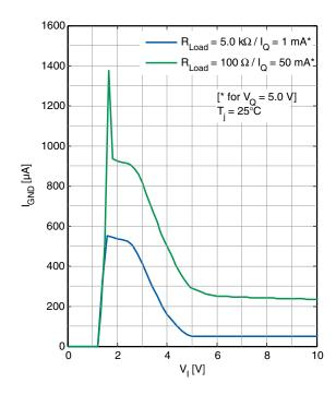
Quiescent Current  $I_q$  versus Input Voltage  $V_1$
