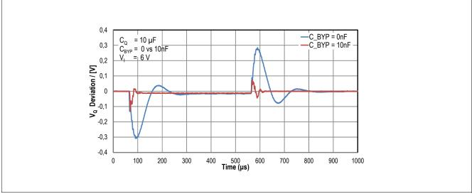
Figure 6 Influence of  $C_{\text{BYP}}$ : example of transient response to one and the same load step with and without  $C_{\text{BYP}}$  of 10 nF ( $I_{\text{O}}$ : 100 mA to 500 mA)
