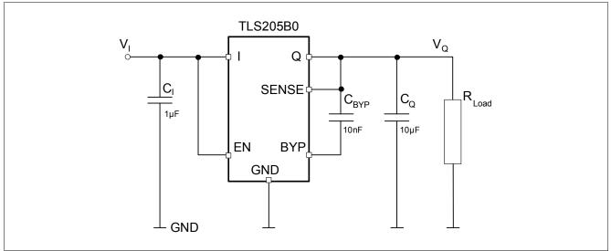
Figure 4 Typical Application Circuit TLS205B0 V50
