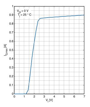
Reverse Output Current versus Output Voltage  $V_{\rm Q}$
