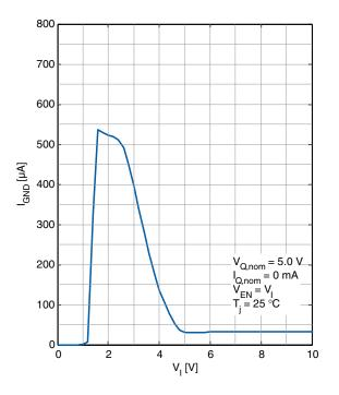
GND Pin Current  $I_{GND}$  versus Input Voltage  $V_1$
