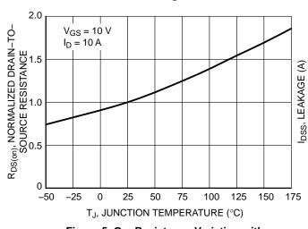
Figure 5. On–Resistance Variation with Temperature
