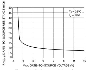
Figure 3. On-Resistance vs. Gate-to-Source Voltage
