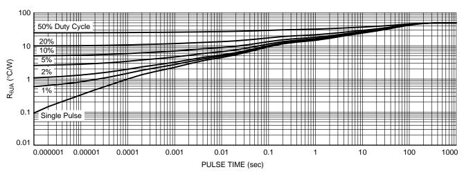
Figure 13. Thermal Characteristics
