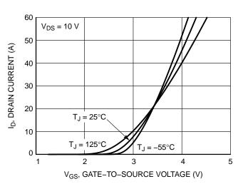
Figure 2. Transfer Characteristics
