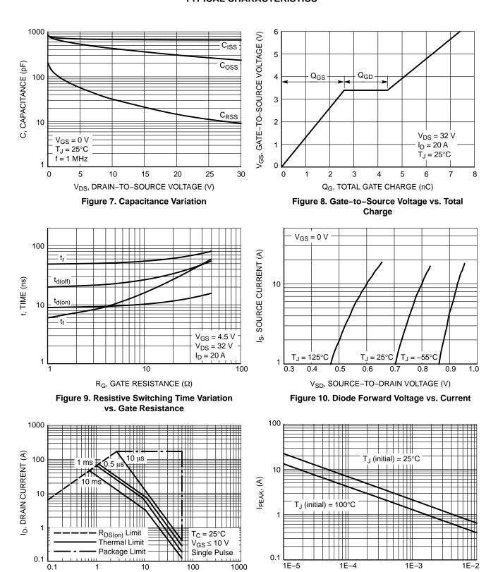
Figure 11. Maximum Rated Forward Biased Safe Operating Area
