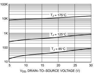
Figure 6. Drain-to-Source Leakage Current vs. Voltage
