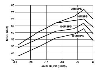
FIGURE 7. SFDR vs AMPLITUDE, f<sub>CLK</sub>/f<sub>OUT</sub> = 5
