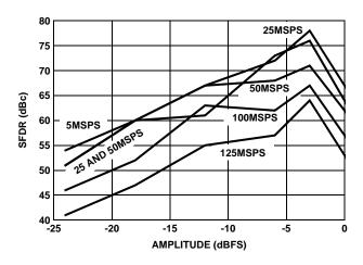
FIGURE 26. SFDR vs AMPLITUDE,  $f_{CLK}/f_{OUT} = 5$
