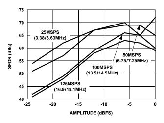
FIGURE 27. SFDR vs AMPLITUDE OF TWO TONES,  $f_{CLK}/f_{OUT} = 7$
