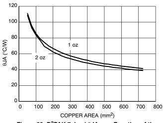
Figure 29. D<sup>2</sup>PAK 7–lead  $\theta$ JA as a Function of the Pad Copper Area Including Traces, Board Material
