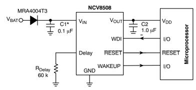
\*C1 required if regulator is located far from power supply filter.
