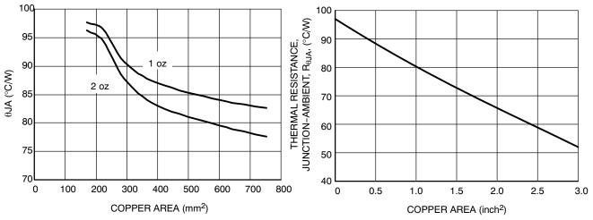
Figure 22. SOIC 16–Lead  $\theta$ JA as a Function of the Pad Copper Area Including Traces, Board Material
