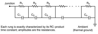
Figure 27. Non-Grounded Capacitor Thermal Ladder ("Foster" Ladder)
