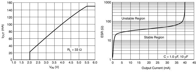
Figure 14. Output Current vs Input Voltage
