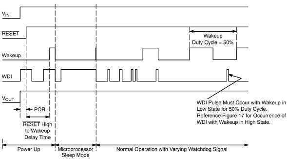
Figure 3. Power Up, Sleep Mode and Normal Operation
