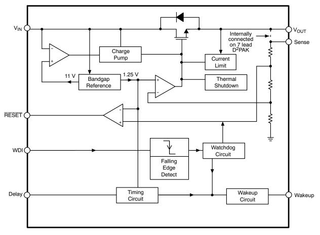
Figure 2. Block Diagram
