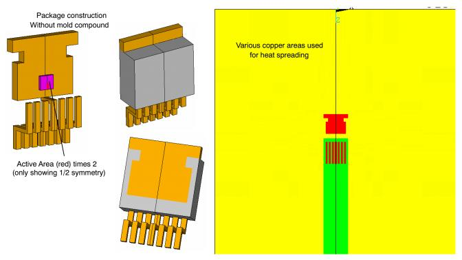
Figure 28. PCB Layout and Package Construction for Simulation
