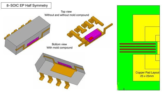
Figure 34. Internal Construction of the Package and PCB Layout for Multiple Pad Area
