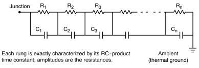
Figure 33. Non-Grounded Capacitor Thermal Ladder ("Foster" Ladder)
