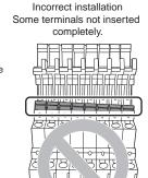
Do not insert short bar in the hole for wire or screw driver, it may cause the result of failure of pull out.
