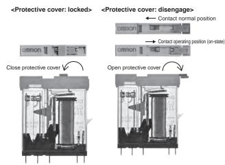
Keep the protective cover open when using the latching lever. Move until the latching lever clicks to the ON position (ON state). After use latching lever, in order to prevent malfunction, return the switch to contact normal position (OFF state), and make sure the protective cover is firmly closed.
