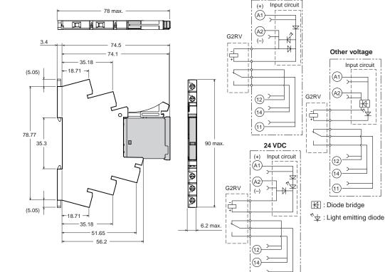
Terminal Arrangement/Internal Connection Diagram
