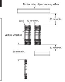
\* When five or more are installed, install with 10 mm space between each.
