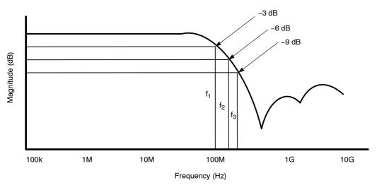
Figure 8. Filter Bandwidth
