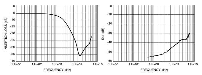
Figure 4. Typical Insertion Loss Characteristic
