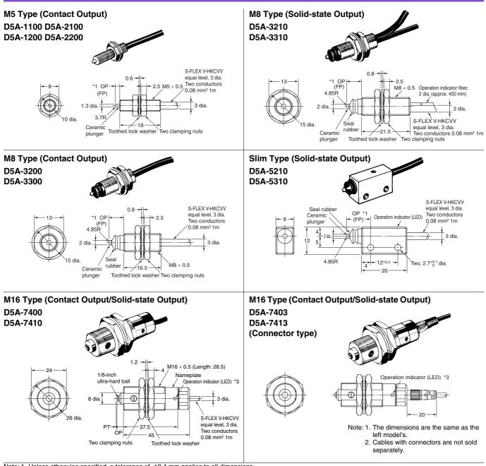
Note: 1. Unless otherwise specified, a tolerance of ±0.4 mm applies to all dimensions. 2. Special screw dimensions apply to the case screws (pitch: 0.5 mm). Mounting is not possible with standard tapping. Use the provided special nuts.
