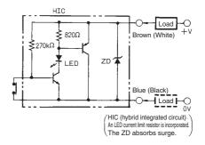
Note: The load may be connected to either the +V or 0 V terminal. Core wire colors have been changed accompanying changes in standards. The old core wire colors are given in parentheses.
