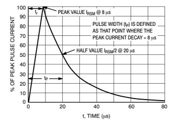
Figure 1.8 x 20 µs Pulse Waveform
