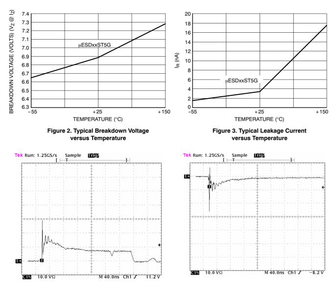
Figure 4. Positive 8 kV contact per IEC 6100-4-2
