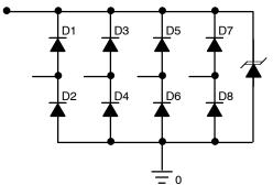
Figure 8. NUP4106 Equivalent Circuit
