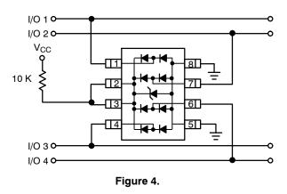
The NUP4106 can be isolated from the power supply by connecting a series resistor between pins 2 and 3 and  $V_{CC}$ . A 10 k $\Omega$  resistor is recommended for this application. This will maintain a bias on the internal surge protection and steering diodes, reducing their capacitance.
