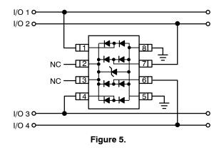
In applications lacking a positive supply reference or those cases in which a fully isolated power supply is required, the internal surge protection can be used as the reference. For these applications, pins 2 and 3 are not connected. In this configuration, the steering diodes will conduct whenever the voltage on the protected line exceeds the working voltage of the surge protection plus one diode drop (Vc=Vf + VRWM).
