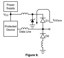
The resulting clamping voltage on the protected IC will be: Vc = VFD1 + VRWM.
