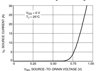
Figure 10. Diode Forward Voltage vs. Current
