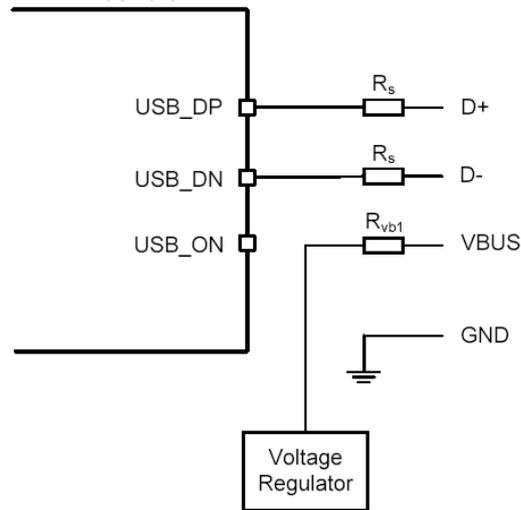
**Figure 23: USB Connections for Bus-Powered Mode**
