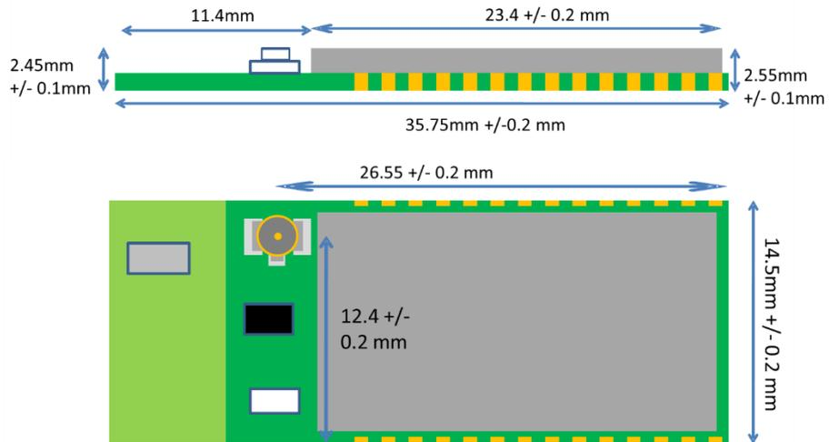
**Figure 11: Dimensions of WT11u-E**
