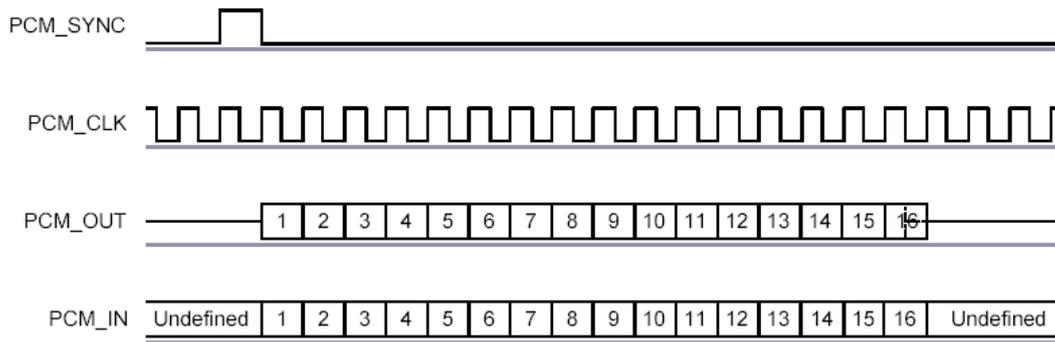
**Figure 28: Short Frame Sync (Shown with 16-bit Sample)**
