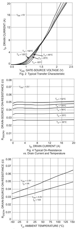
Fig. 6 On-Resistance Variation with Temperature
