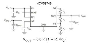
Figure 16. Typical Application Schematics
