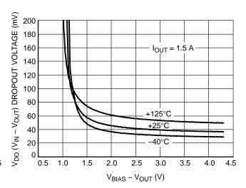
Figure 7. V<sub>IN</sub> Dropout Voltage vs. I<sub>OUT</sub> and Temperature T<sub>J</sub>
