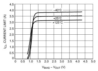
Figure 15. Current Limit vs. ( $V_{BIAS} - V_{OUT}$ )
