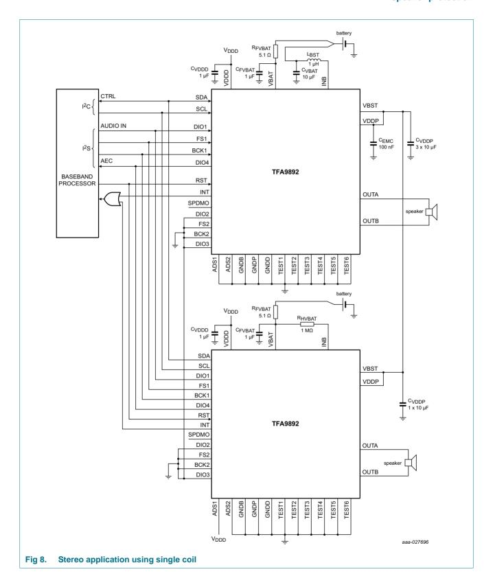
12 V boosted audio system with adaptive sound maximizer and speaker protection
