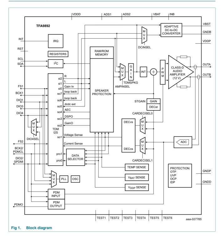
12 V boosted audio system with adaptive sound maximizer and speaker protection
