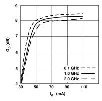
Figure 3. Power Gain vs. Current.
