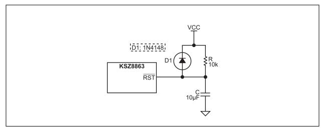
Figure 8-2 shows a reset circuit recommended for applications where reset is driven by another device (for example, the CPU or an FPGA). At power-on-reset, R, C, and D1 provide the necessary ramp rise time to reset the KSZ8863MLL/FLL/RLL device. The RST\_OUT\_N from the CPU/FPGA provides the warm reset after power-up.
