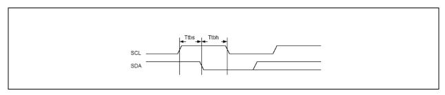
FIGURE 7-11: I<sup>2</sup>C STOP BIT TIMING
