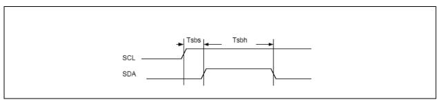
FIGURE 7-12: I<sup>2</sup>C OUTPUT TIMING
