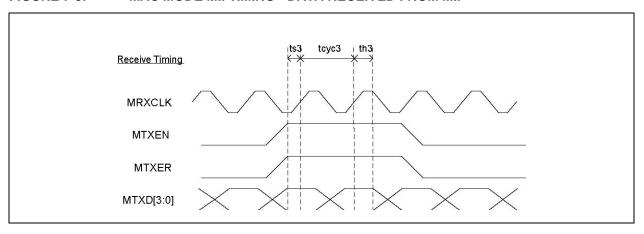
FIGURE 7-4: MAC MODE MII TIMING - DATA TRANSMITTED TO MII
