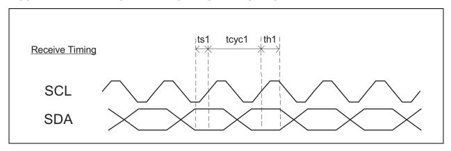
FIGURE 7-2: EEPROM INTERFACE OUTPUT TIMING DIAGRAM
