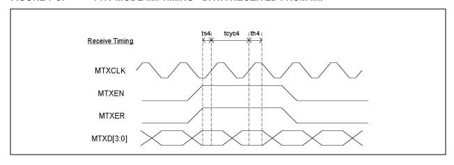
FIGURE 7-6: PHY MODE MII TIMING - DATA TRANSMITTED TO MII
