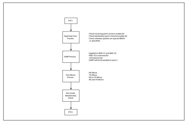
FIGURE 3-5: DESTINATION ADDRESS RESOLUTION FLOW CHART, STAGE 2
